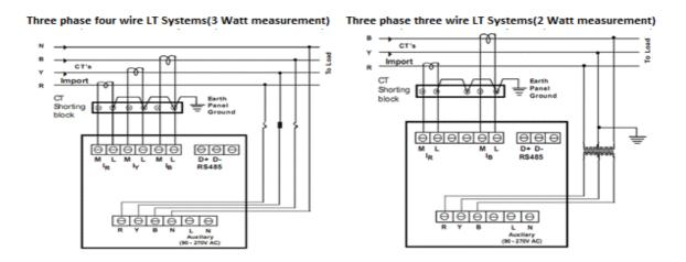
The test terminal box (TTB) is basically provided inside the enclosure of the metering box. It is basically a wiring arrangement to provide for testing the meter and also to isolate the meter from the instrument transformer secondary connection.
